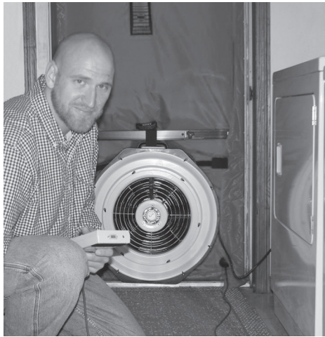
Home Energy Auditor conducting an air leakage test with a blower door.
