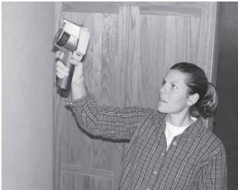
Homeowner demonstrating use of IR camera to check for insulation voids and air leakage paths.
